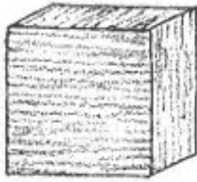
Fig. 130. Striations on a pyrite crystal show that the structure does not have all the symmetry operations of a cube.
